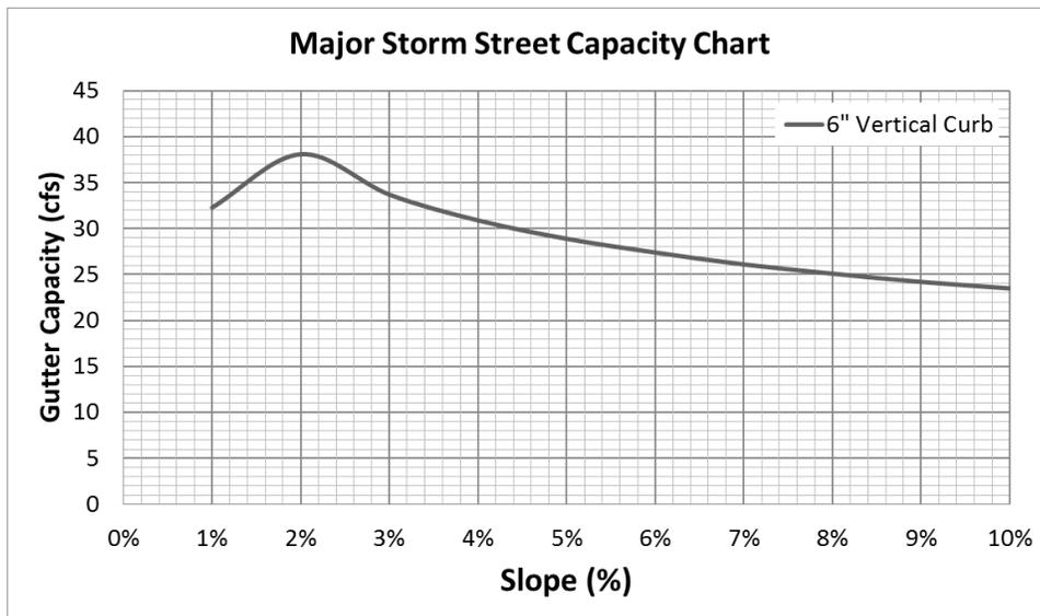
**Figure 7-1. Street Capacity Chart Local Type I**
