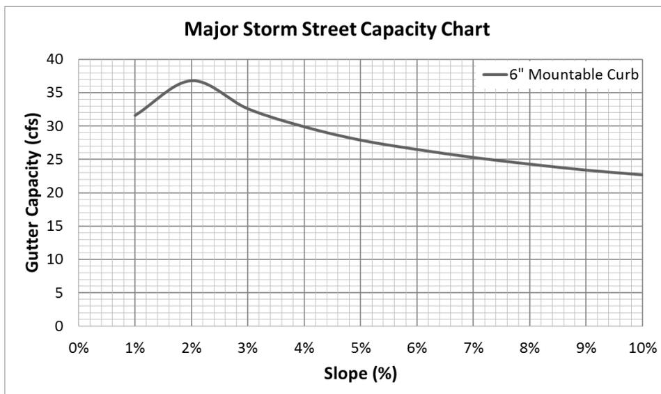
**Figure 7-2. Street Capacity Chart Local Type II**
